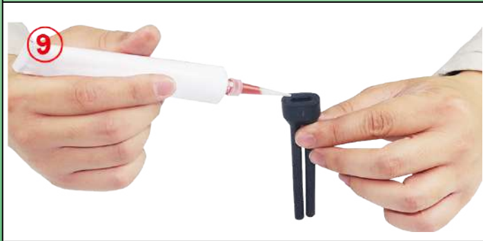
9: Pour silicone resin (RTV) in the wires input hole of the silicone boot
