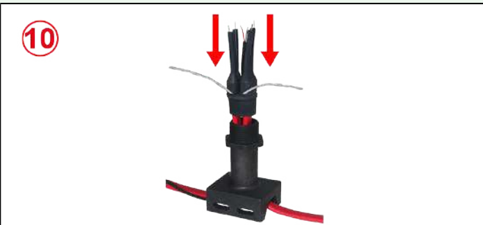
10: Slide the insulating sleeves over the conductors of the heating cables, leaving the ground conductor outside.
